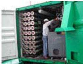
OZONE ON BOARD. A container on the deck of the Tonsina (above) houses canisters of ozone (below). Mueller/Nutech-03; Stubblefield/ENSR International
